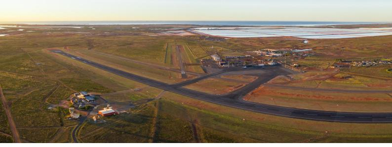
The 6 month project ran concurrently with the installation and testing of the new Medium Intensity Runway Lighting infrastructure. The taxiway construction was cement stabilised using fine crushed rock over cement-stabilised pindan, with a code 4E foundation strength requirement.
